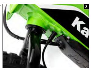
\* Using the provided adapter, the battery can be also charged from a car, camper or SxS vehicle with a 100-110 V AC power source, making it easy to charge up for the next ride while away from home. (Charging time will vary depending on the available amperage.)
