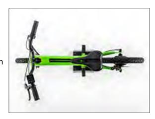
\* Adjustable seat height is 410 mm at the lowest and 520 mm at the highest, accommodating 3- to 8-year-olds between 95 and 140 centimetres and under 45 kg. (Photo 10)
